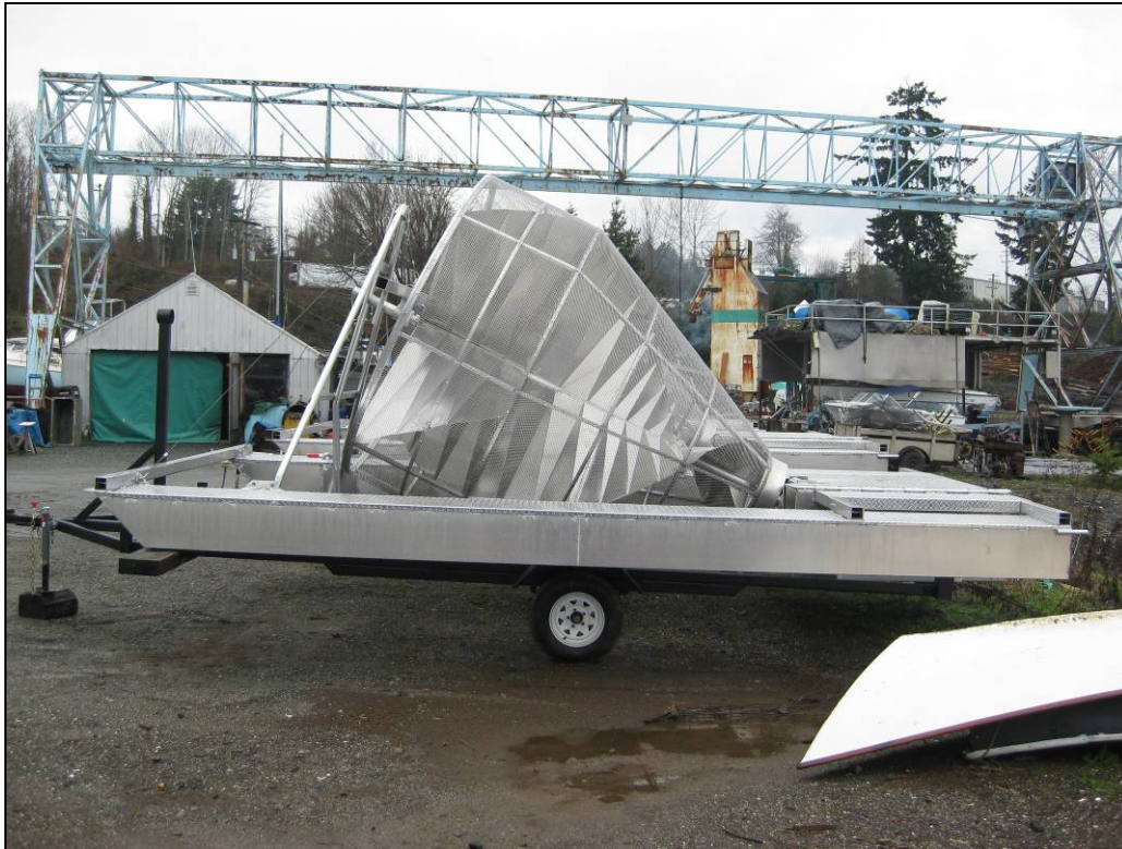
Photo 1. Photo of a rotary screw trap that will be used in the Peace River sampling program.
